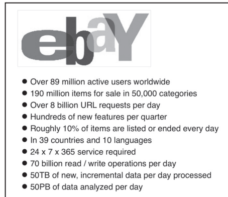
Figure 5.1 Statistics that show why sites such as eBay can't survive with a centralized database. That database must be partitioned into multiple databases. Partitioning (or sharding ) is a critical strategy for scaling.
