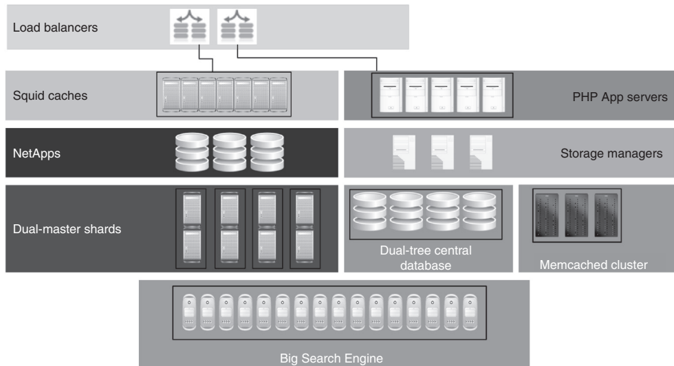
Figure 5.8 Flickr's architecture includes many levels. First is load balancing as incoming connection requests arrive. Squid caches are open-source web-delivery systems that operate as reverse proxies for HTML pages and images. The PHP App Servers connect to the shards and keep the data consistent. The storage managers do the actual mapping from an index to the correct shard. NetApps are for mass storage of photos. Their fundamental database architecture uses dual masters for each shard. This gives them resilience in the case of failure. The dual-tree structure is a custom set of changes to MySQL that allows scaling by incrementally adding masters without a ring architecture. The central database includes data, such as the users table, which includes primary user keys (a few different IDs) and a pointer to which shard a user's data can be found on. The Big Search Engine is a replication of the database Flickr wants to search.
